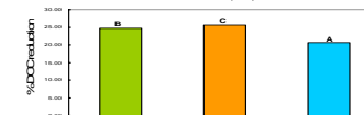
Fig. 3 Reduction in dissolved organic carbon (DOC) of humic samples after 4 weeks irradiation.
