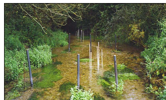
Measuring exchange of nutrients between the surface and subsurface zones in the River Lambourn
